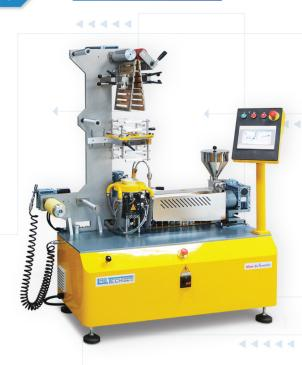
Our Mini Scientific Single-Layer Film Blowing Line is a practical choice for R&D in film-blowing applications with its compact design taking up little floor space offering an economic alternative for a quality control line of masterbatches. This line features a Mini 16 mm Single-Screw Extruder, a Spiral Mandrel with a 25 mm annular die lip diameter for uniform film blowing production, and an easy-to-use computerized LCD touchscreen control panel.
