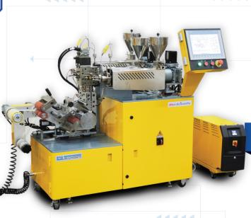
Our Mini Scientific 3 & 5 Layers Co-Extrusion Cast Film Line is designed to provide a compact laboratory-scale solution for researching and developing new cast films. This line features 3 units of Mini 16 mm Single-Screw Extruders for producing film with 3 or 5 layers. It is also equipped with a 5-Layer Feedblock which can be configured to A-B-C or A-B-C-B-A film layer structure and can also be optionally equipped with a Weighing Hopper for precise feeding.
